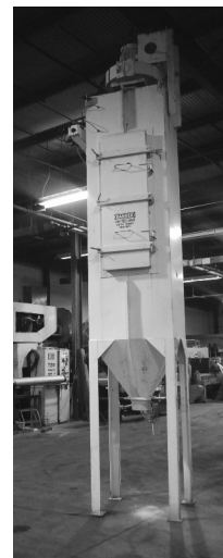
York 7 1/2 HP Bag House Dust Collector
