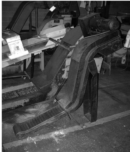
Jorgenson Chip Conveyor
