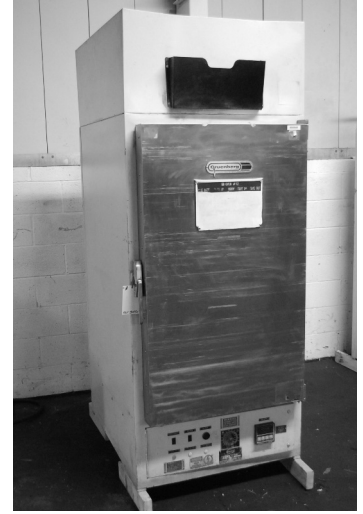
Gruenberg 150° C Electric Oven
