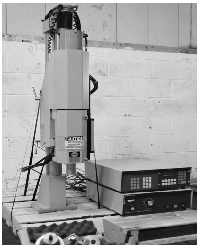
Sonic & Materials 2,500 Watt Ultrasonic Plastic Welder
